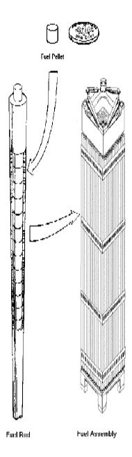
This sketch illustrates how the pellets make up a rod and how the rods, in turn, are grouped together to form the fuel assembly.
